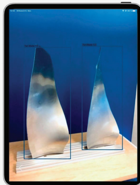
Camera live view with predicted damages
