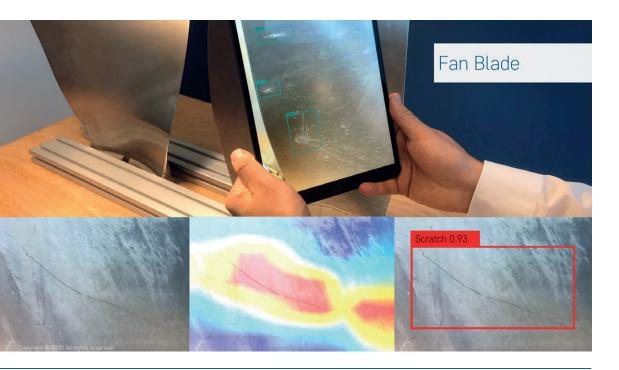
**Al2Go** reliably identifies different damage types simultaneously in one picture. The process involves image processing, damage identification, classification and the output of the inspection result.
